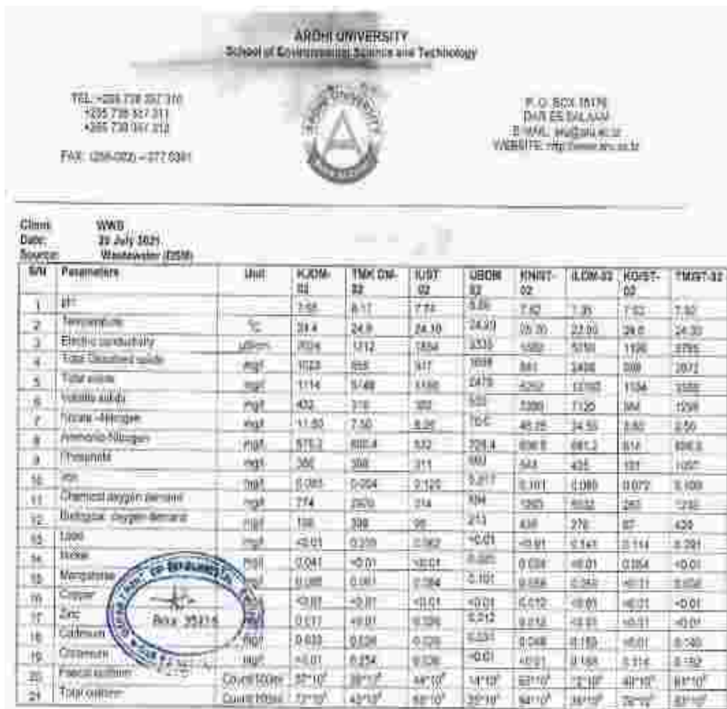
Figure 4.1 Water quality test results (Source Design Report 2021)
